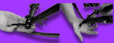
**Note**: the rear & front brake discs should be aligned on the same side
