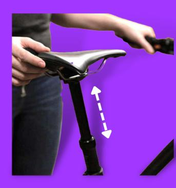
6.3 Lock the seat post to the frame using the quick release provided
