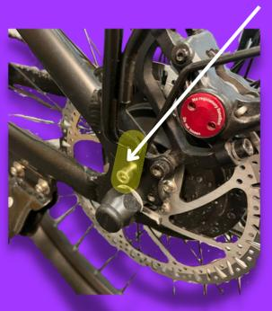
9.3 Make sure that the left rear screw is tightened to the upper hole in the rear frame (not the bottom hole). The same things needs to be done at the right rear side of the bike
