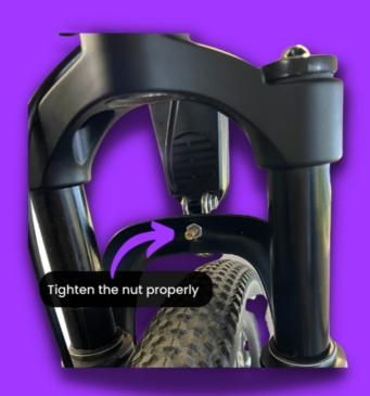
4.2 Ensure that the nut is tightened so that it does not remain loose
