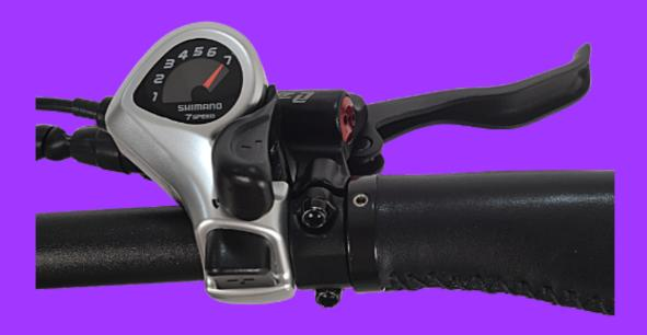
For best experience, use lower gears like 1 or 2 when climbing uphill (riding at lower speeds) and use higher gears for flat surface (riding at higher speeds)
