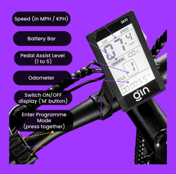
Switching ON/OFF the monitor: Press M button for 2 seconds
